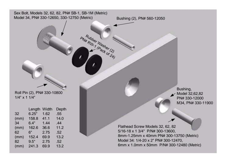
Once a solid flat surface has been prepared for the magnet, it must be positioned so that its face is parallel and centered to the strike plate. When the magnet has been experimentally positioned this way, it's ready for mounting.
